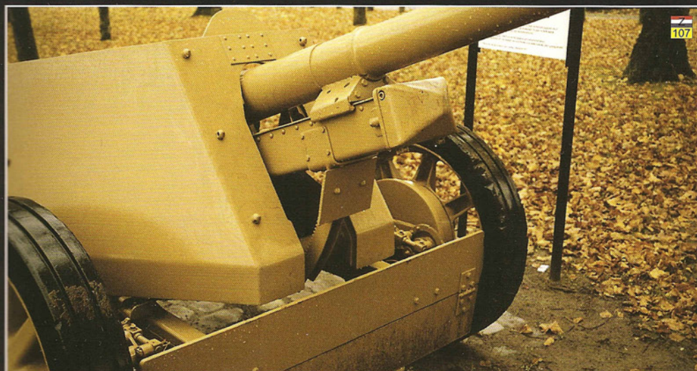
107 The gun in Zandoerle is fully elevated; the top of the sliding armour emerges from the top of the gun shield. The lower gun shield is not original. This one has only two hinges, whereas the original has four.
