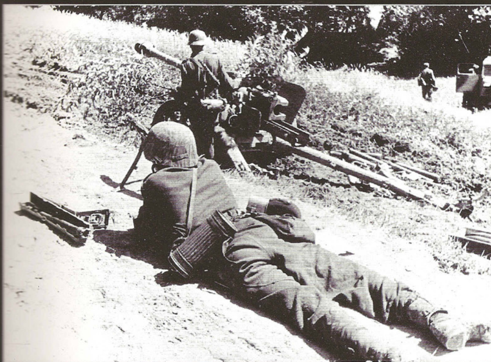
[Left] A PaK 40 in the position next to a road. Empty cartridges are gathered next to the trail of the gun so as not to be underfoot. These would be collected to be reused or melted down. One of the gunners is still adding branches to camouflage the gun. Its tow vehicle is further down the slope. Single color camouflage over dark yellow is visible on the door. The machine gunner is wearing a helmet cover issued from 1942 onwards, though never as widely as with the SS. Note the open container with the spare barrel for the machine gun. [Zbigniew Lalak Collection]
