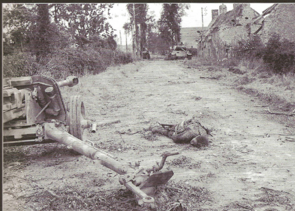
[Left] A knocked-out German 7.5 cm anti-tank gun and one of its gunners lying dead beside it. A disabled Panther tank is visible in the background. This PaK 40 has received camouflage that appears to have been sprayed on. Note the vertical container for the Sprengpatrone Z 72 demolition charge. Fontenay-le-Pesnel, Normandy, 25 June 1944. [Photograph B5939 courtesy of the Imperial War Museum, London].
